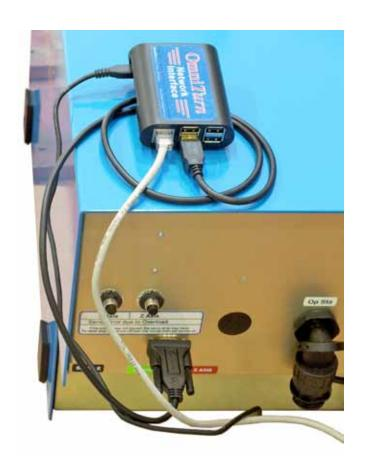
The network interface acts as a bridge between the Omniturn's RS232 port and the network (via WiFi or Ethernet).
