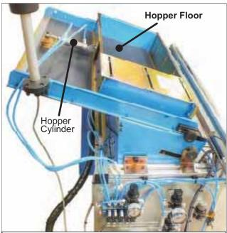
Typical air line routing, wide hopper
