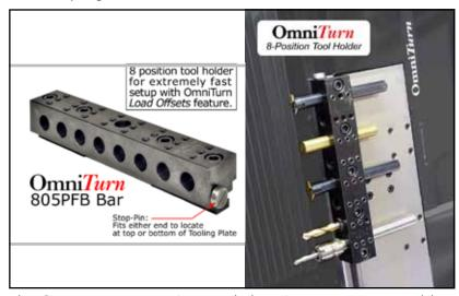
The OmniTurn 805PFB (pictured above) is an 8-station tool-bar that accepts 5/8" tooling on 1.1" centers. Stop-pin fits either end so bar can be located on either side of OmniTurn tooling plate. OmniTurn "Save Offsets" feature instantly retrieves offsets when program is loaded, so repeat jobs can be re-set in minutes. Shown at right on OmniTurn GT table note that steep 75° angle allows chips to fall away quickly into chip-pan.
