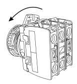
Typical BACO: rotate tab to left to remove contact block assembly from panel-mounted operator.
