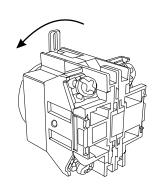
Typical IDEC: rotate tab to left to remove contact block assembly from panel-mounted operator.
