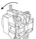
Typical IDEC: rotate tab to left to remove contact block assembly from panel-mounted operator.
