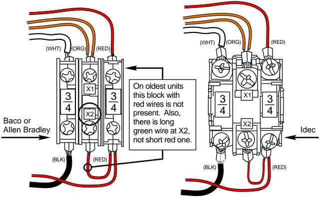
**NOTE:** The very oldest units will have GREEN wire at X2, not RED jumper, and no contact block at the right, if so **leave that block empty on the new switch**.
