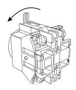
Typical IDEC: rotate tab to left to remove contact block assembly from panel-mounted operator.
