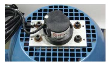
The encoder is mounted on a plate which has been centered on the sub-shaft at the factory. Do not loosen the four 1/4-20 socket-head screws which fasten this plate to the fan housing. Do not loosen any of the screws that hold the fan
