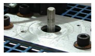
The encoder shaft has two flats milled at right angles. There are two corresponding set-screws on the encoder. Carefully slide the encoder onto the shaft, being certain that the set-screws line up with the two flats in the shaft.
