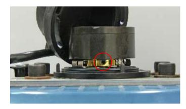
Use a 0.050" hex wrench to tighten the two set- screws. Hold the encoder assembly flush against the mounting plate while tightening the set-screws.
