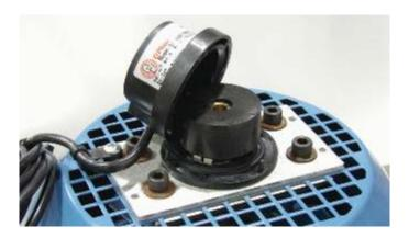
Fold the encoder cover over the encoder and fasten with two 6-32 socket-head screws (supplied). Fix the cable-tie strain relief to the shaft using supplied hardware.
